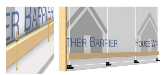
**Step 9:** Insert the trimmed rainscreen board into the row of starter clips. Gently tap board with rubber mallet if need to insert the board fully into the clips.
